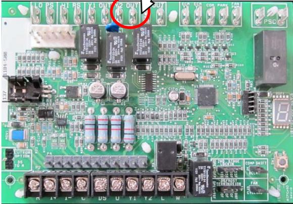
**Figure 14. K4 Compressor Modulating Solenoid**
